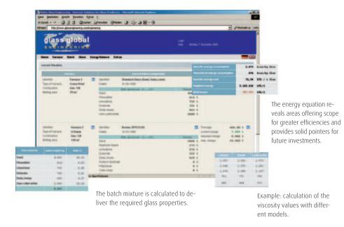
For the optimisation of batch composition management, the program allows for the saving and management of batch compositions, silo set-ups and evaporation rates. It provides an extensive material database, containing default values for glass compositions that can be supplemented with specific settings.
