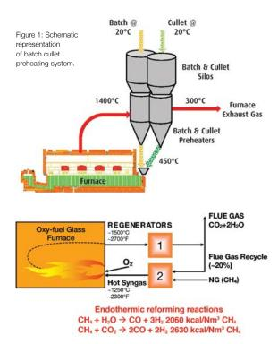
Figure 2: Schematic representation of OPTIMELT TCR Process.
