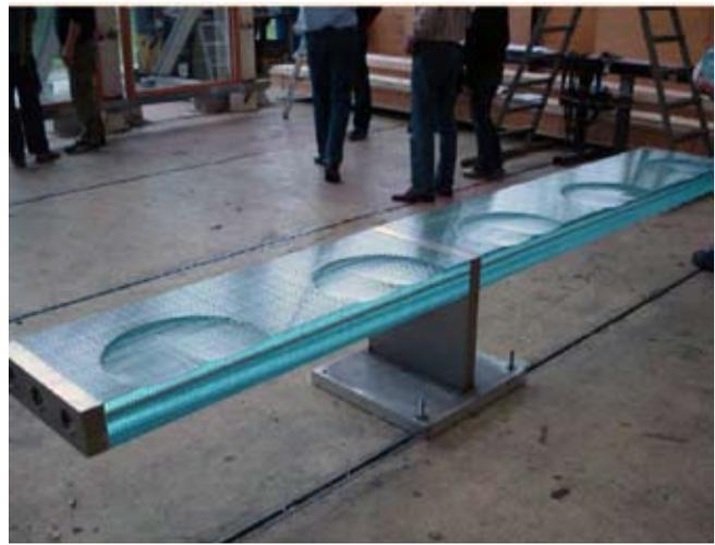
These bridge constructions all have the inherent redundancy of a polycarbonate interlayer that, in the case of massive glass breakage (no pane remains whole), the bridge still supports its designated live load – although in a sagging geometry more like a rope bridge.
