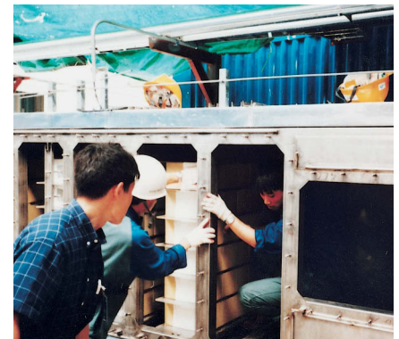
DeNO x system for glass melting process, 21,000 m 3 /h
