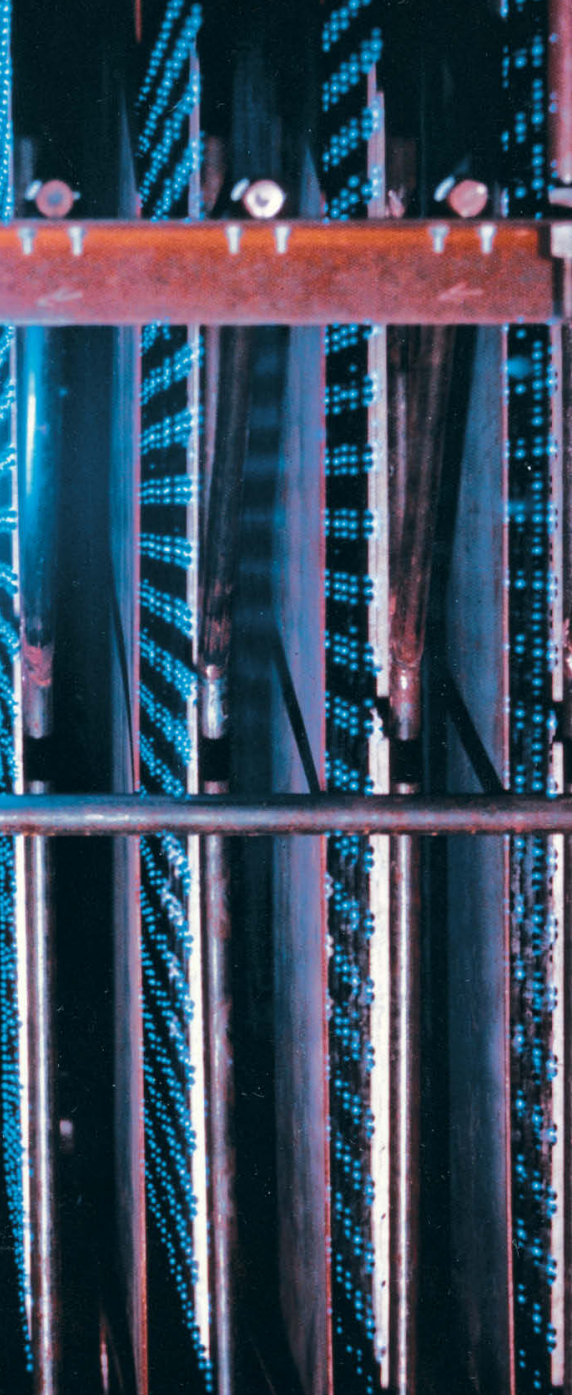
Vertical wet electrostatic precipitator for aerosol separation in the plastic industry
