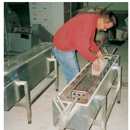
Mobile trail catalytic plant with catalytic soot filter and DeNO x catalyzer, waste gas volume 500 Am 3 /h. The trial plant can be equipped with up to 3 rows of DeNO x - or oxidizer elements.
