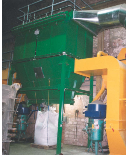
Cartridge filter for a sand blasting plant 40,000 m 3 /h
