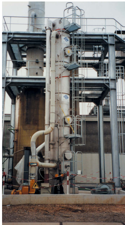
Mobile trial wet absorber / wet electrostatic precipitation plant, waste gas volume 2000-3000 m 3 /h. This plant is equipped with complete EMSR technology and can be fitted with various wet absorbers.
