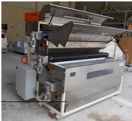
Minerali Industriali uses and provides complete magnetic separation plants. MAG-3 separators have been specially designed by Minerali Industriali to remove main paramagnetic minerals thanks to 3 high field separation stages built in an extremely compact implementation at the same time easily accessible for maintenance.
