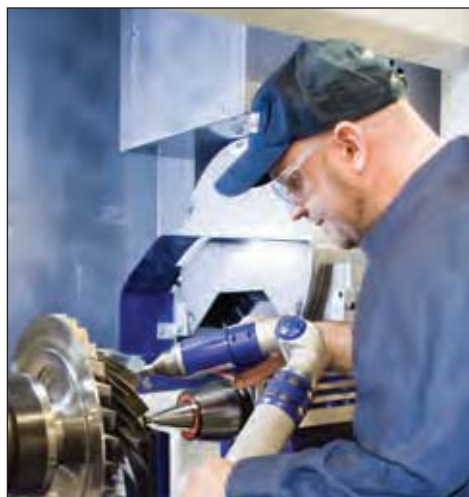
High performance five axis milled impeller profiles are authenticated with a digital coordinate measuring machine.
