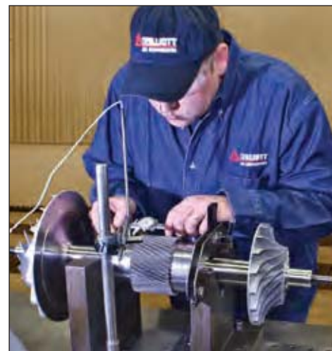
Precision built high-speed rotor assemblies are dynamically balanced and documented in accordance with API 672 standards.
