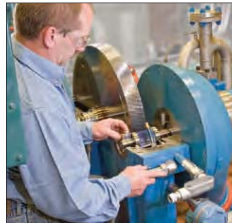
The bearing top half can be taken off after removing two screws. The bottom half of the bearing can be rolled out and removed from the casing for inspection. The two-piece seal assembly can be removed by sliding it into the bearing cavity area; then follow the same procedure that was utilized for removing the bearing.
