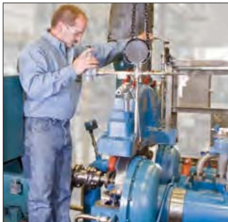
Gear case cover lifts off easily, exposing gears, bearings, and seals – without removing any other components.
