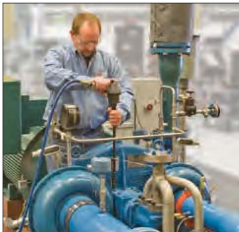
Easily accessible bolting facilitates the removal of the gear case cover.
