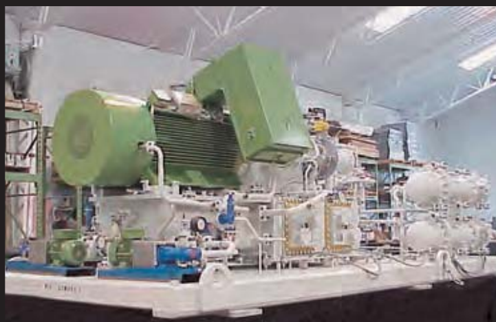
This Engineered Air, 2,670 CFM (4,540 m 3 /hr) system was designed for a Middle East Oil refinery. This air package design was based on API 672 plus comprehensive EPC and End User specifications. This compression unit is applied for the production of unleaded/low sulfur gasoline.
