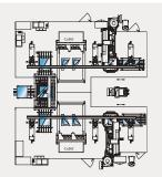
**B'CHAMP QL VARIANT 1** Increased capacity with two cells and fully integrated pre-cutting
