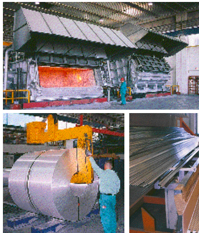
Above: Aluminium ingots are loaded into a moulding furnace and fed out as 4mm strip, kept in 2 metre diameter rolls. Pressed again to 3 microns thick, strips are made into spacer bar on nine-station forming machines, packed with care by hand and boxed in stillages ready for delivery
