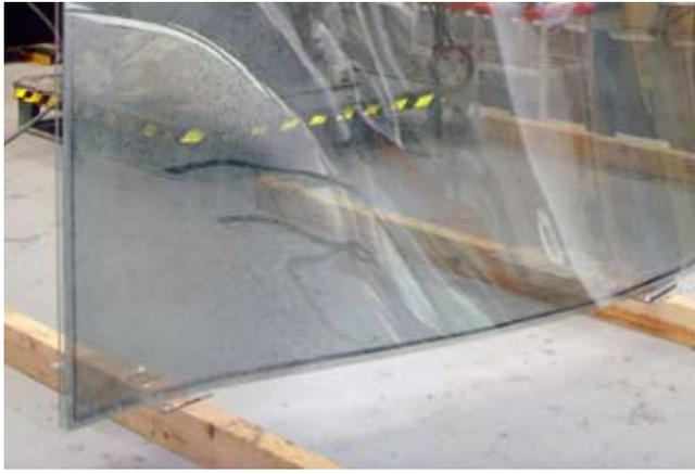
sealant cures sufficiently for the IG unit to be handled. Glass handling devices such as vacuum cups, straps, etc. are used to transport the assembled IG unit as appropriate.
