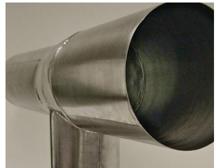
Fabricated chamber made of iridium sheet
