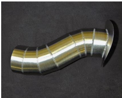
Fabricated tube made of platinum/rhodium sheet
