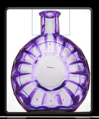
Defect detection possible **around and inside** the engraved areas.
